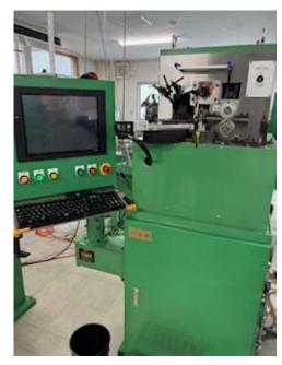
Traditionally, achieving high-load springs required increasing both the width and thickness of the material, which in turn necessitated a larger coil diameter. However, our newly developed equipment dramatically improves the rigidity of key mechanical components, enabling the production of springs that can withstand high loads even with a small diameter.
